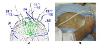
**Fig. 2.** Ultrasound probe compatible device. The distance between two adjacent probe positions is 50mm, and the angle between two adjacent probes is  $40^{\circ}$  in unbent situation. (a) Diagnosis method for the belt-shaped device. (b) Clinical experiment for the belt-shaped device on a patient.
