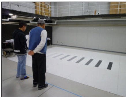
Fig. 8 The 2nd experiment Visibility of line of different luminance contrasts
