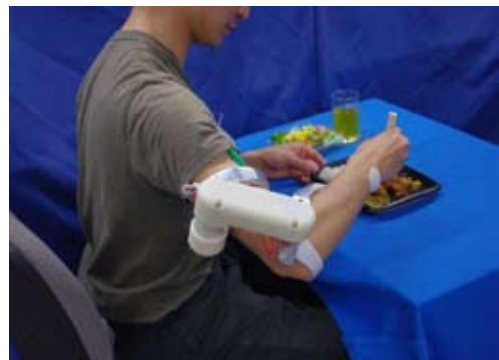
Fig. 1 Wearable robot for patients with essential tremor
