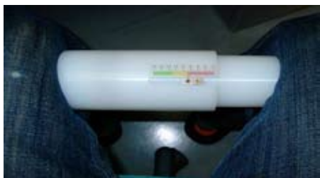
Fig. 3 Knee-gap force measurement device
