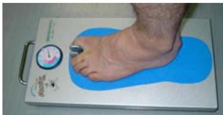
Fig. 2 Toe-gap force measurement device
