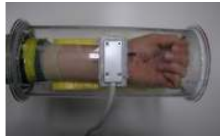
Fig. 1 An air-tight chamber developed in the present study.
