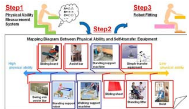
Fig. 1 Algorithm for selecting appropriate transfer support equipment based on the physical ability of the user
