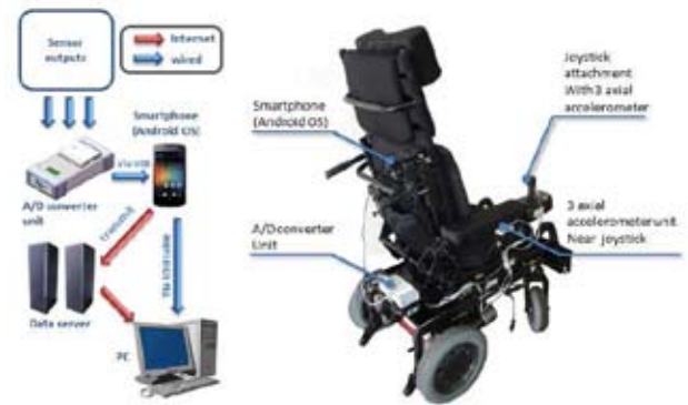
Fig.1 Schematic of WELL-SphERE and Sensors and system Set up position
