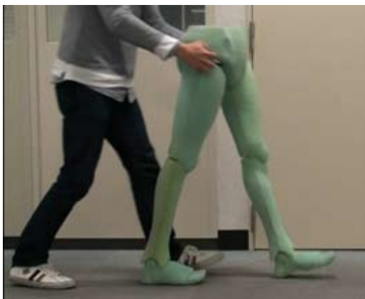
Fig.1 Biped anthropomorphic passive walker
