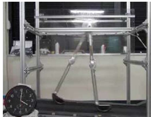
Fig.2 Non-stop walk for 27 hours on a treadmill
