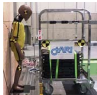
Fig. 2 Collision between a child dummy in front of a wall and a moving object.
