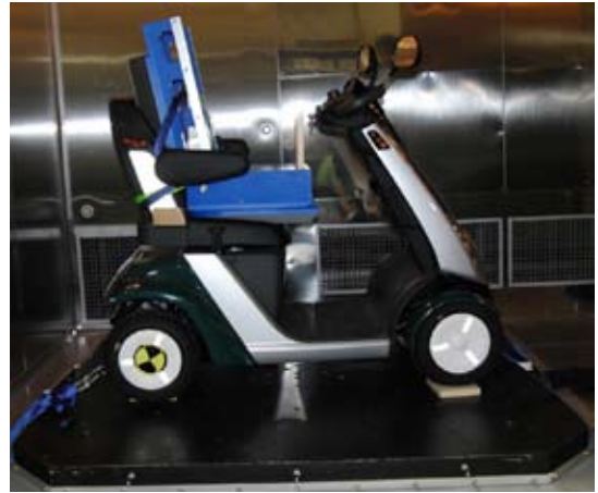
Fig. 2 Electrically powered scooter vibrating vertically
