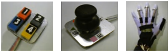
(a) Push switch (b) Joy stick (c) Sensor glove Fig. 7 Input interfaces
