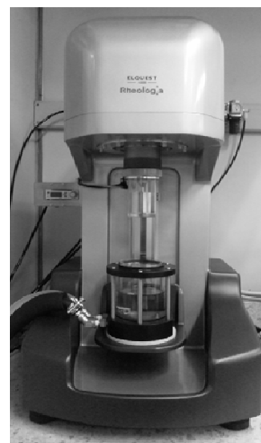
Fig.1 Observation and cross-section of the shearing portion of a double-cylinder type rheometer
