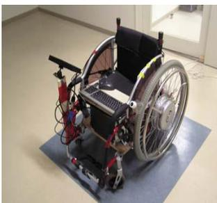
Fig. 1 Electric power-assisted wheelchair (JW-II)
