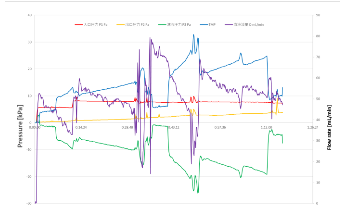
Fig.7 Pressure of DP6 centrifugal pump
